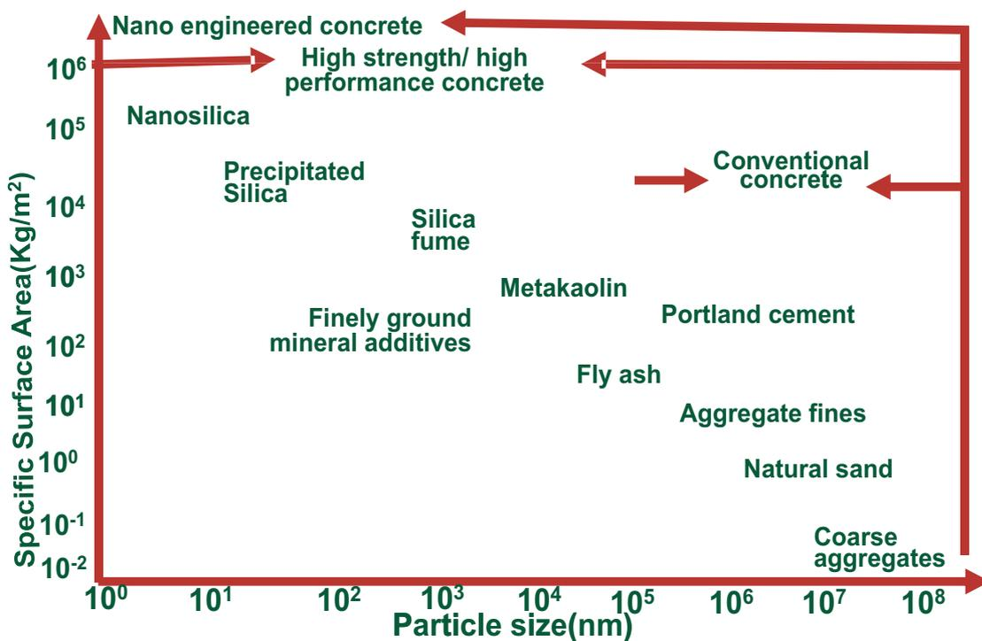
⇒ Nanoparticles allow better void filling & positive filler effects & improved bond between pastes aggregates; nanosized additives increase strength beyond what is attained with conventional materials
