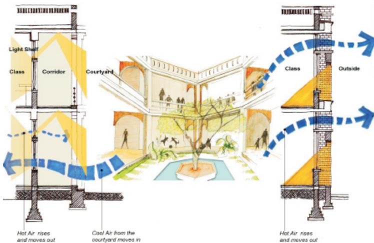
The courtyards are proportioned to be shaded and are also cooled using the principle of evaporative cooling with water. These courtyards also let in diffused light into the classrooms.
