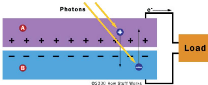
**Figure 1. Operation of a photovoltaic cell**
