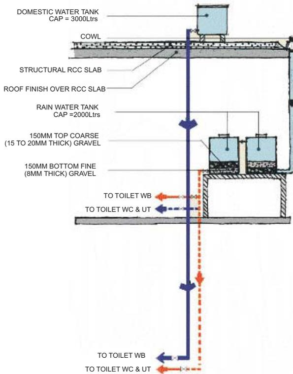
Rainwater harvesting & Wastewater reuse: Not just occurring but “visible”
