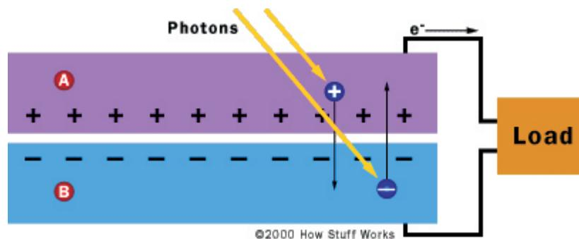
Figure 1. Operation of a photovoltaic cell
