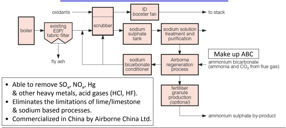
Saleable products: (NH<sub>4</sub>)<sub>2</sub>SO<sub>4</sub>; NH<sub>4</sub>NO<sub>3</sub>; NH<sub>4</sub>HCO<sub>3</sub> (with CO<sub>2</sub> capture)
